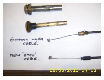
It is critical that the nipple end is a good fit in the choke control lever. My efforts to source a new cable were not successful, so I tried the local bike and motorbike shops. Having met with no success there, I tried the local garden machinery service centre. The nipple size and shape for an ATCO Motor Mower is exactly the same as my 1937 Opal. The only difference being the outer cable having a different diameter on the end to be used next to
